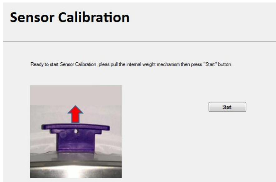
Pull the internal weight handle as shown on the above picture and press 'Start', scale will display –PUSH–
