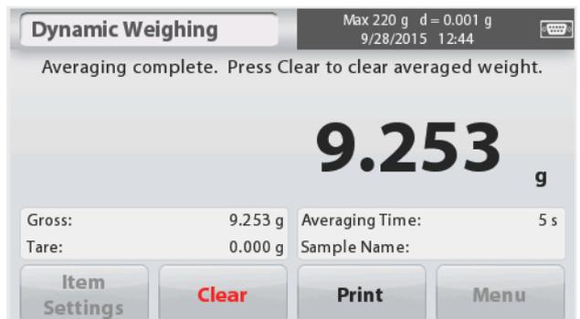
**Note:** Clear the pan before beginning a new Dynamic Weighing cycle.
