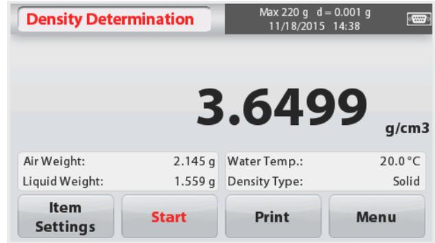
Press **Start** to reset all the weight values and restart the process.
