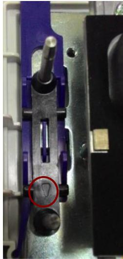
Up close of the weight holder (Note the position marking on the holder which facing scale front end when installing back in position.
