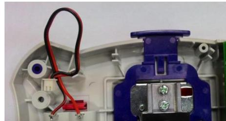
Detach battery compartment connector and set it aside.
