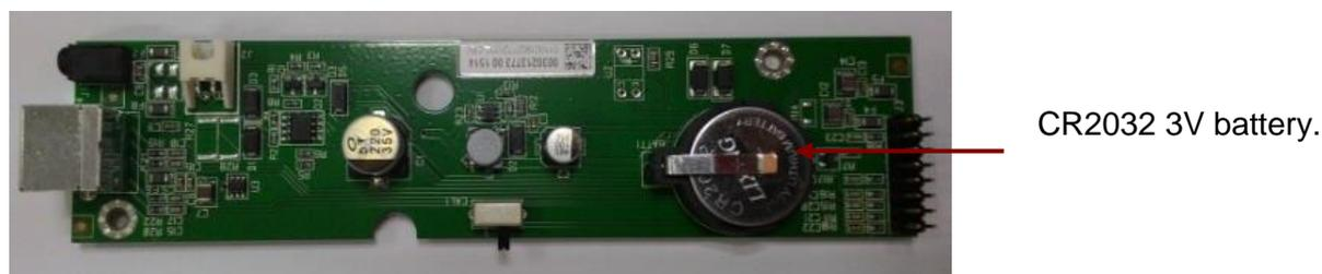
**Note:** Once the Power PCBA is removed from the main PCBA scale date and time will reset back to factory default.
