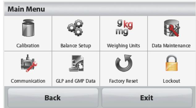
When the Security Switch is in locked position, the Calibration and Lockout menus will be hidden.
