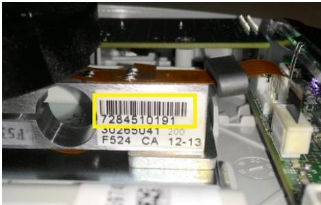
For scale which the load cell has never been replaced before you can obtain the load cell serial number on the load cell itself as shown on the right side picture (example 7284510191)
