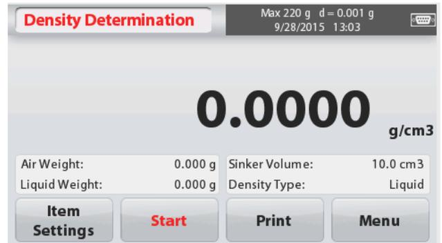
**Step 1 of 2 – Weigh the Sinker in Air.**
