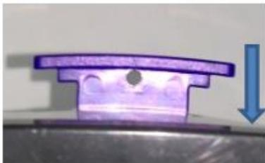
Wrong handle position during PUSH. (Only halfway not fully close scale).
