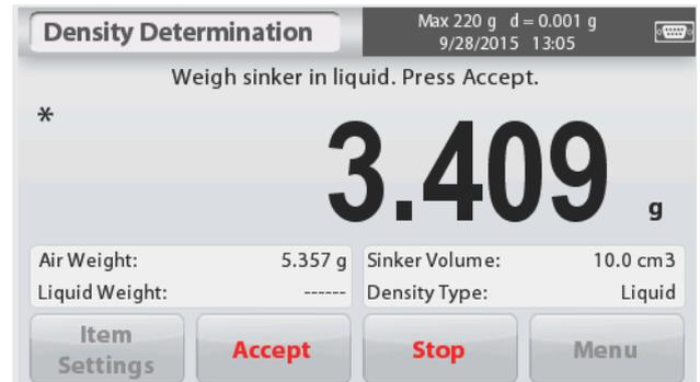
Once the necessary weights have been determined, the density of the Liquid sample is displayed in **g/cm<sup>3</sup>**(along with the weight in air, weight in water) on the Application screen.
