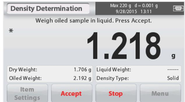
Once the necessary weights have been determined, the density of the sample is displayed in **g/cm<sup>3</sup>** (along with the weight in air, un-oiled and oiled, and weight in water) on the Application screen
