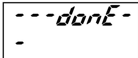
When calibration finishes, **Done** appears briefly, and the scale returns to weighing mode displaying the weight on the weighing pan.
