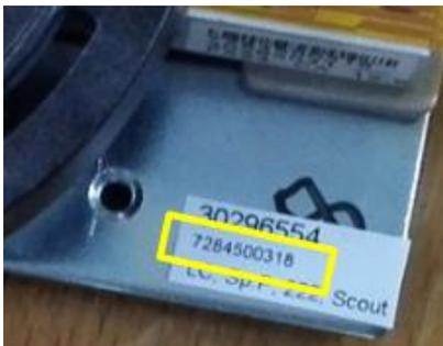
For scale which the load cell had been replaced before you can obtain the load cell serial number on the load cell label as shown on the right side picture (example 7284500318)
