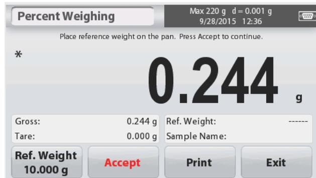
Alternatively, press the **Ref. Weight** button from the Percent Weighing Recalculate Ref. Wgt screen to establish a new reference weight manually through a numerical keypad. Key in the desired Reference Weight, then press **Save**.
